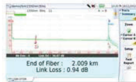
Fig. 27 Example of results trace with Smart Test
