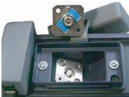
Fig. 16 Position of the adapter onto the connector
