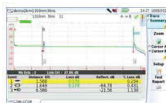
Fig. 29 Trace + Table results in Smart Test
