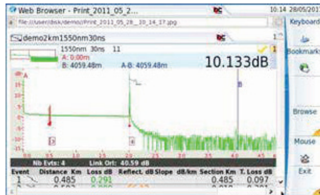
Fig. 84 Example of screenshot, open in the Web Browser of the FiberXpert OTDR 5000
