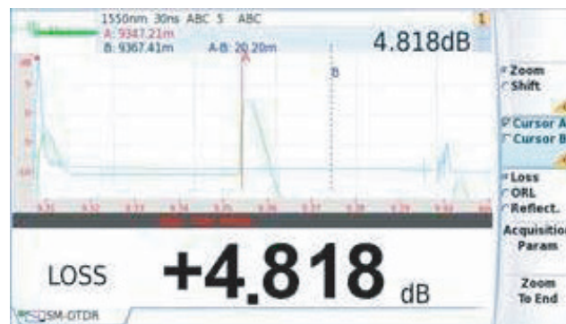
Fig. 26 Example of loss measurement
