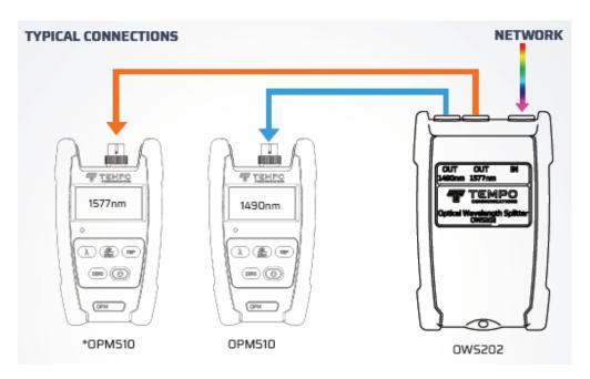
The loss of the OWS200 has negligible effect on the measurements as the OWS loss is typically less than 0.1dB. In the above example the OPM510 used to measure 1577nm is set to 1550nm. Errors due to not measuring at the exact wavelength are small since the typical responsivity of an InGaAs OPM is very flat over the 1530 - 1625nm range.
