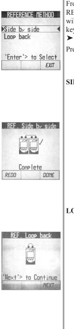
From the Autotest Main screen, press the REF softkey. The Reference Method screen will be displayed. Use the UP/DOWN arrow keys to highlight ➤ SIDE BY SIDE ◄ or ➤LOOP BACK ◀.
