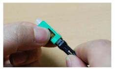
10. Press the connector shell towards the fiber to release the bending fiber.
