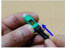
Make sure the assembly jig is on the connector. Insert the fiber into the connector.
