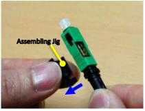
9. Remove the assembly jig.
