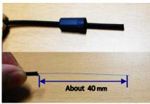
2. Install the boot & strip off 40mm of the cable jacket.
