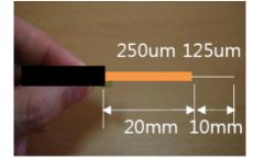
Prepare the fiber for a total lenght of 30mm (20mm of acrylic coated fiber and 10mm of bare fiber with a cleaved end) as shown on the packing bag label.
