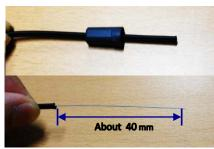
2. Install the boot & strip off 40mm of the 3mm cable jacket and 900 micron buffer.
