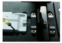
5. Insert cleaving fixture into the 920CL and cleave the fiber.
