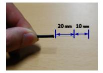
Fiber should now be identical as shown above as 20mm of acrylic coated fiber and 10mm of uncoated fiber wit a cleaved end.
