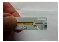
Lay the cable into the cleaving fixture. Twirl the kevlar strand and insert into the hole as shown.
